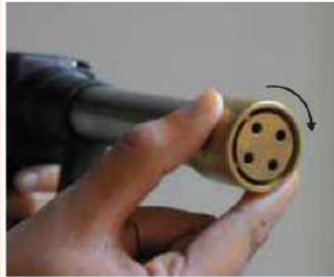
Fine spray to fight close range Class A fires such as fires in wood, paper and cloth, and electrically started fires.
