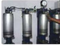
✓ Hydro Static Pressure Test
